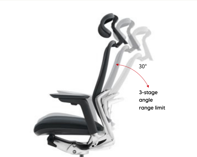
Recline The backrest can be locked and unlocked by turning the left lever under the seat assembly. The maximum tilt angle is 30°, and has the function of locking the initial angle and 3-stage angle range limit.
