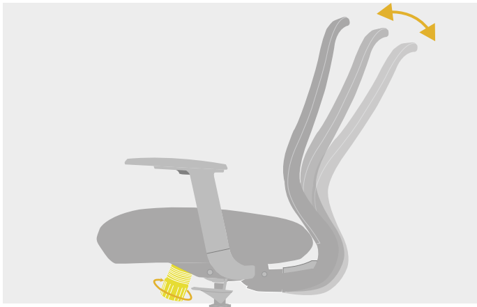
Tilt elastic adjustment gear, adjustment range 20 degrees
